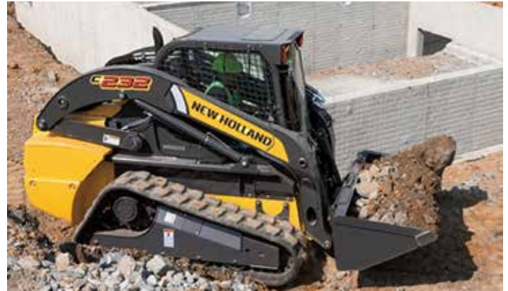
An example of a New Holland construction compact track loader, offered by KBE
